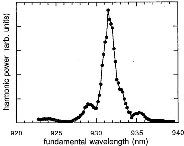
FIG. 1. Wavelength tuning curve for room-temperature single-pass SHG of a Ti:Al<sub>2</sub>O<sub>3</sub> laser in periodically poled LiNbO<sub>3</sub>.
